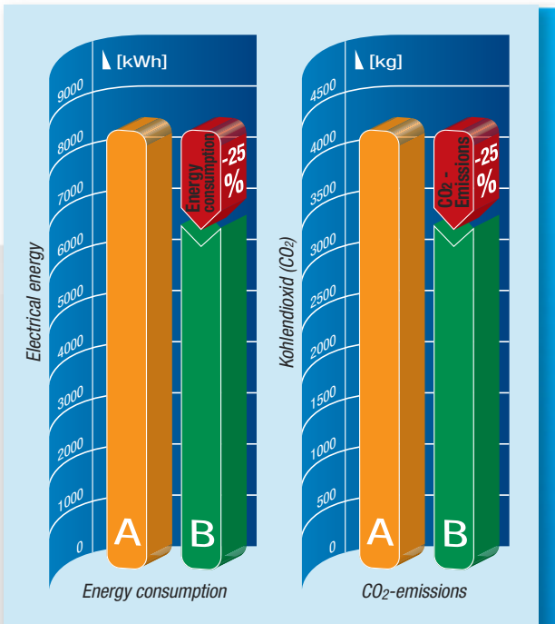
Fig. 1: Annual energy consumption and CO 2 emission when charging a 48 V – 500 Ah traction battery (240 charges per year) A: Conventional charger B: BELATRON high-efficiency charging system
